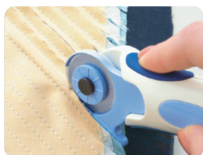
Insert into a channel between two stitching lines and push forward.
