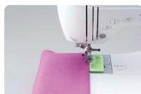
Top Stitching: place the guide in front of the presser foot and sew.
