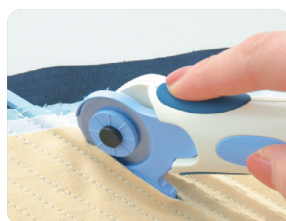
Fabric will be cut as you push the cutter forward.
