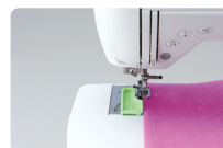
Top Stitching: place the guide in front of the presser foot and sew.
